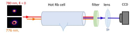
The experiment uses a rubidium two photon transition to realize a four wave mixing process generating a blue radiation (@420 nm) as output from an input excitation @780 and 776 nm. The setup uses a hot cell of rubidium vapor illuminated by adequate laser beams, and allows examining the vortex transfer from red laser beam (@776 nm) to blue.
